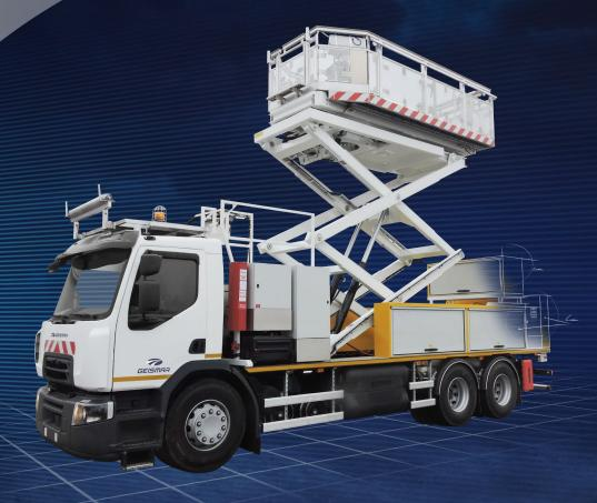
Safe and performant solution for urban catenary maintenance and adjustments Bi-mode motorization for cleaner and quitter operation Bogie technology and safe on-tracking Easy handle of railway equipment
